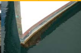
Dirty boat as seen from above water – poses a biosecurity risk and requires cleaning.
