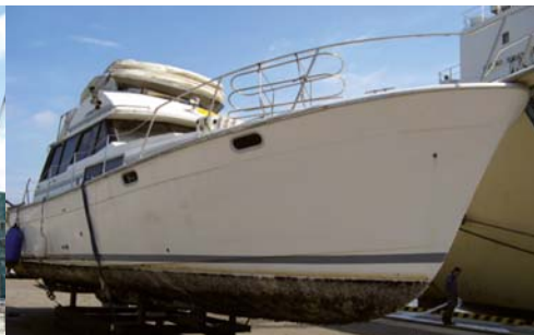
Moderately fouled hull – needs a clean. Fouling organisms already present and fertile ground for marine pests to take hold.
